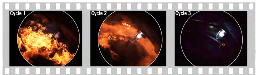
Soot formation in a GDI engine during first cycles of cold start at fixed crank angle
