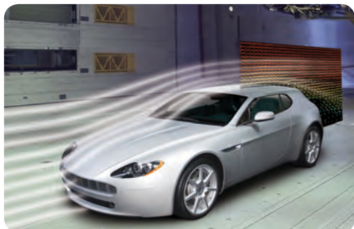
Large 3D flow field imaging in a passenger car wake flow using Helium-filled soap bubbles and time-resolved Particle Tracking Velocimetry (PTV)
